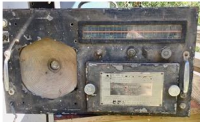
SW/MW Valve Receiver
