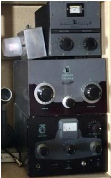
Johnson Viking HF AM CW Tx C/w Antenna 'Matchbox', AM Modulator, Mic and VFO.
