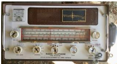
Weston Marine Tx/Rx AM 12v working (80/40m xtal or DDS for Tx)
