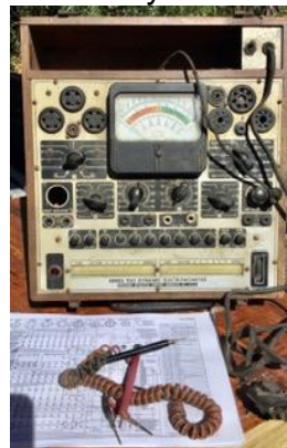
Valve tester for restoration
