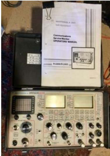
Motorola Test Station OK but Spec Analyser screen not working (a Cap needs replacing)
