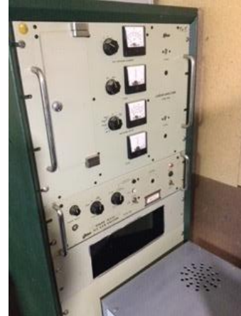
Codan HF Linear Amp complete 4 x 4cx250Bs ex RFDS
