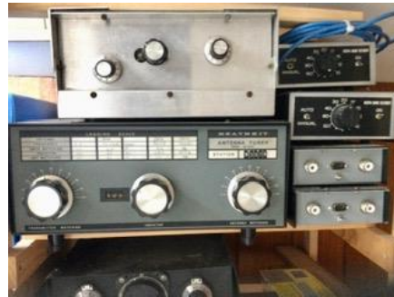
Antenna Matching units and Filters
