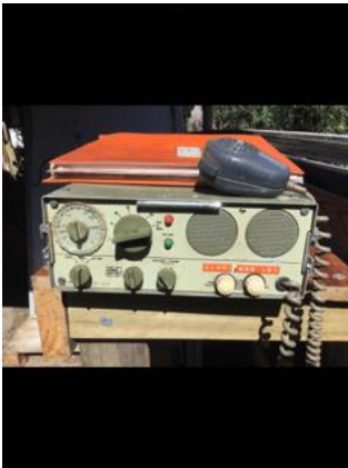
SSB/AM 35w Ship to Shore Tx/Rx with handbook cct
