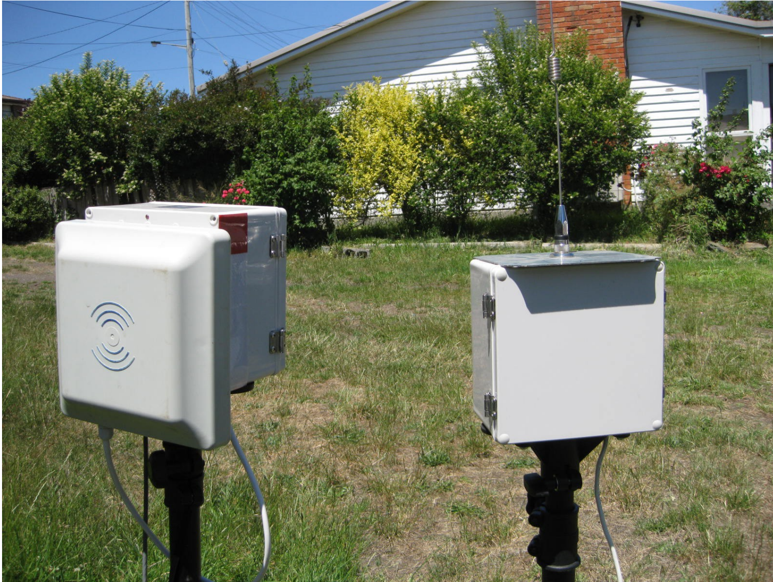
Typical checkpoint setup: 235 x 235mm reader panel with 5 M cable to transceiver unit which has a simple ground plane antenna.
