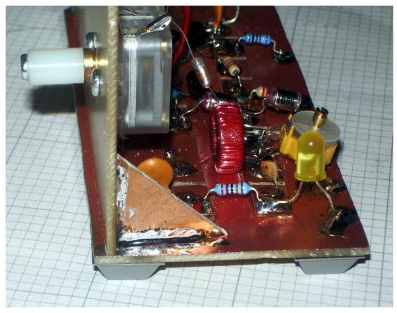
Photo 4 – supporting triangle soldered in place a few mm back from front
