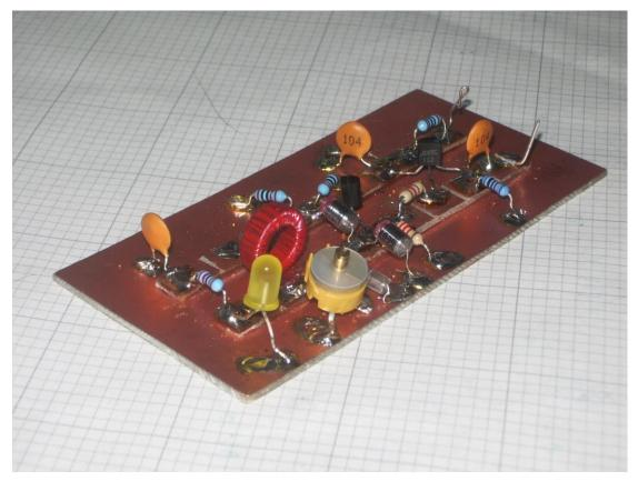
Photo 3 – main 'PCB' components fitted
