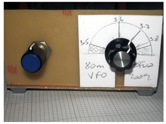
Photo 6 - Front view of completed VFO with 'rough & ready' calibration.
