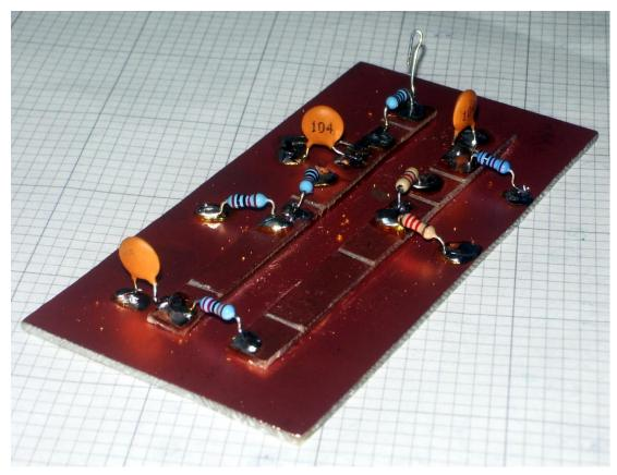
Photo 2 – Components soldered to the islands and ground with short leads
